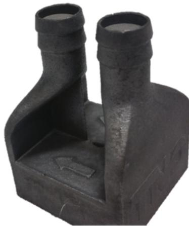
Figure 19: Aluminum alloy pixel AISi10Mg
