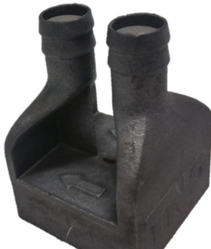
Figure 3: Aluminum Pixel (AlSi10Mg).
