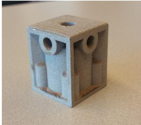
Figure 18: Stainless steel cooling jacket
