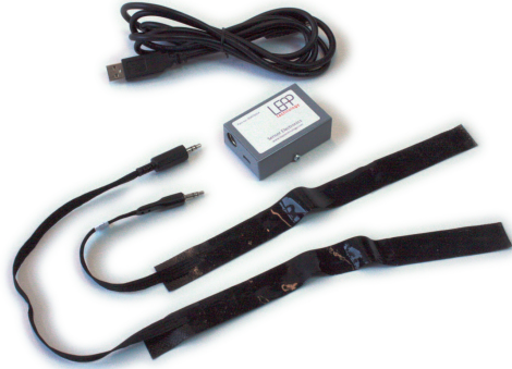
Figure 4.2: Leap technology's stretch sensor evaluation kit with two sensors and the interfacing box [37]
