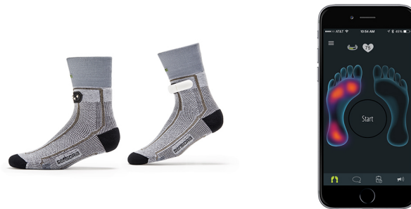
Figure 2.2: The Sensoria fitness sock with the accompanying app showing a heatmap of weight distribution on the foot [13]
