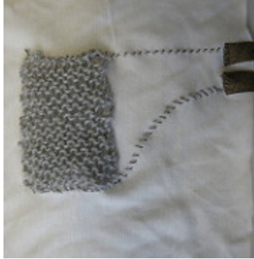
Figure 4.6: Hand-knitted stretch sensor attached to a stretchable fabric with sewn connections for crocodile clamps [43]
