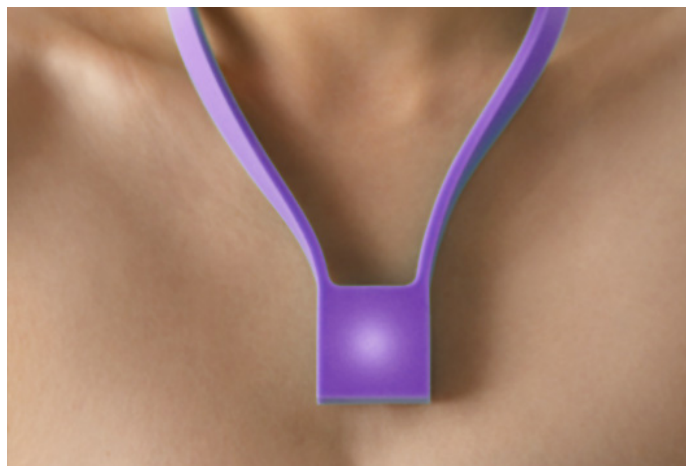
Figure 2.3: The Phillips Vibe necklace emotion sensor showing the emotions of others with the colour of the LED [25]
