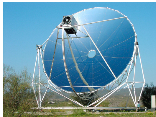
Figure 2 Dual axis parabolic dish CSP system (Quaschnig, 2010)
