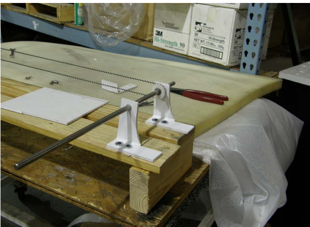
The redesigned brackets did work and kept their shape
