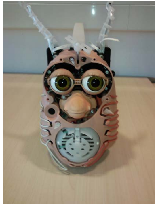
The Furby without the fur. The wires are antennas
