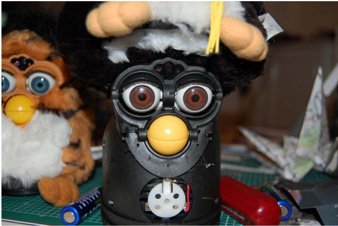
Figure 6.5: A Furby showing its plastic hull
