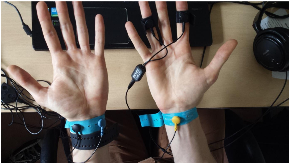
Figure 3. Participant wearing the E4 wristband, the ProComp Infiniti EMG, EKG and finger band electrodes
