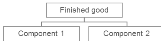
Figure 3-2 One level BOM structure
