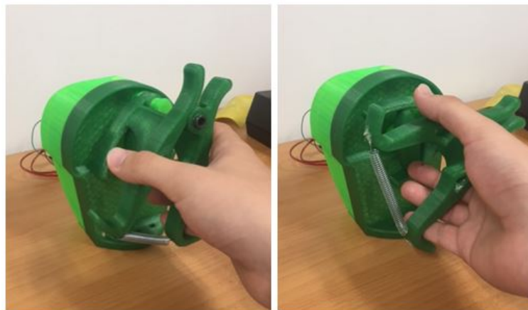
Figure 8.6: Grasp/release and pronation/supination movement generated by the Add-on 2 using the cam. (1) Closed position, (2) P/S, (3) start opening the cam and (4) G/R.
