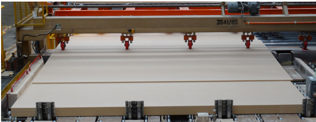
Figure 5.9: Infeed block 133 mm used for sawing board with a length of 4050 mm.
