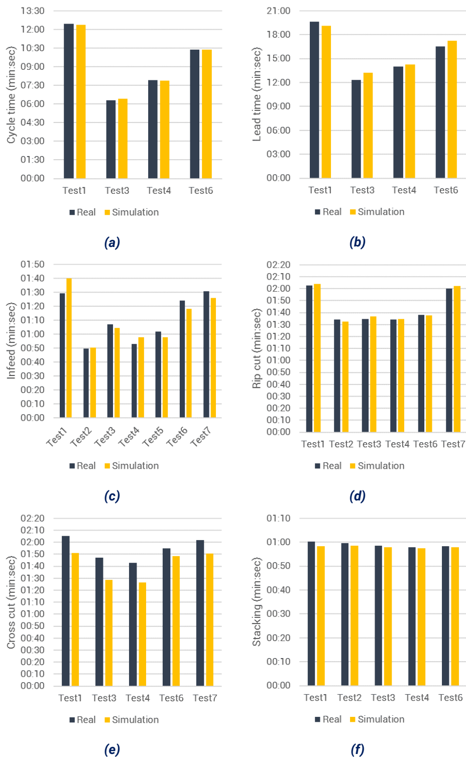
Figure 6.4: Process time comparison between the B-saw and the simulation of the B-saw. The cycle time, lead time, infeed time, rip cut time, cross cut time and stacking time are compared.
