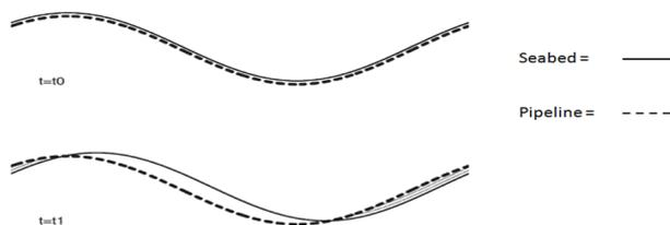
Figure 1-5: Pipe in free span due to migrating sand waves (Morelissen et al., 2003).
