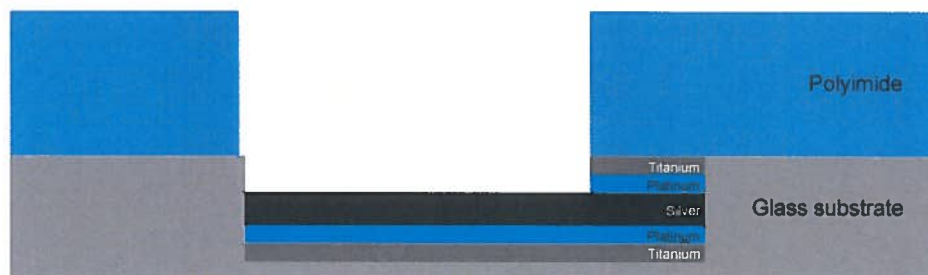
Figure 3.2: Cross-section of the structure of the chip design. Shown thicknesses are not drawn to scale.
