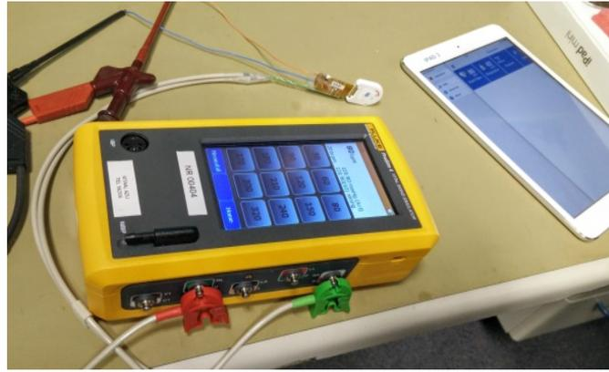
Figure 6 – The experimental setup overview shows the Fluke ProSim 4 patient simulator (front left) the disassembled HealthPatch (centre) and the iPad mini (right).
