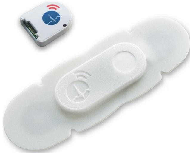
Figure 1 – The HealthPatch MD wearable studied in this thesis is a sensor system consisting of an adhesive patch (left) and a sensor module (right), which is inserted into the patch upon activation.
