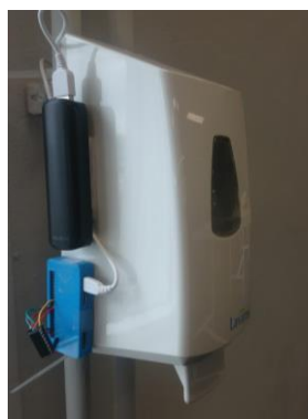
Figure 6. IoT prototype for the soap dispenser.
