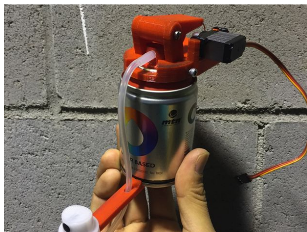
Figure 6: 3d-printed spray-can actuator 8 .
