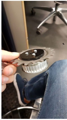
Figure 30: Pulley attached to 19 teeth bike gear.
