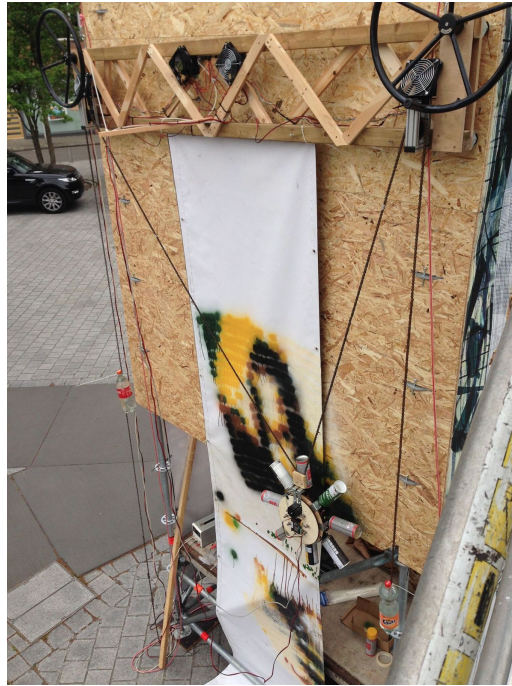
Figure 39: Robot drifting to the right.
