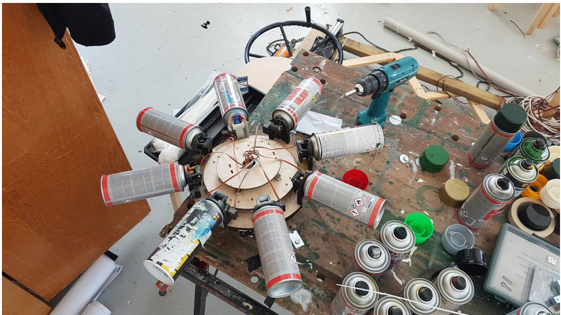
Figure 35: Plotter head with spray-paint cans attached.
