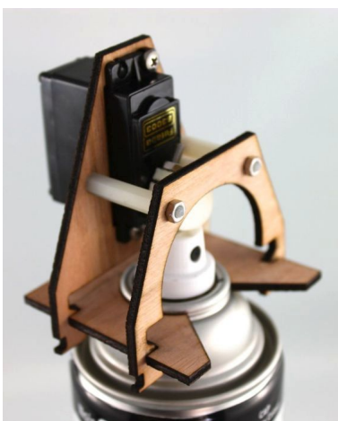
Figure 5: Laser cut spray-can actuator 7 .
