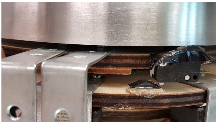
Figure 16: Calibration end-stop of plotter head.
