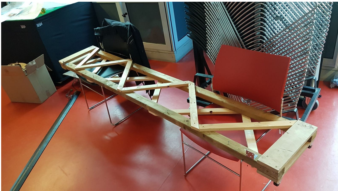
Figure 32: Wooden frame where the motor mounts mount on.
