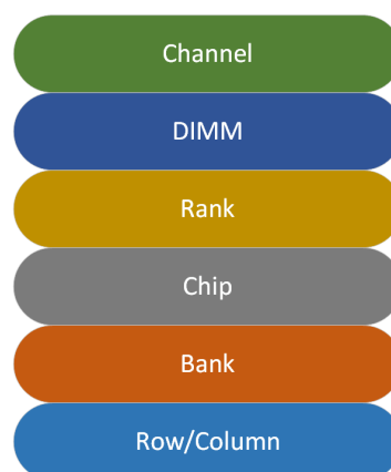
Figure 3.8: Dual In-Line Memory Module memory subsystem organisation
