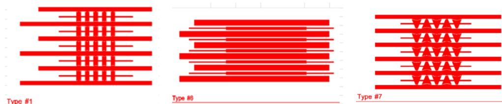
Figure 9: *The three membrane stacks that are used. Left: Type 1, also called the 'original' shape. Middle: Type 6, also called the 'full' shape and Right: Type 7 also called The 'tilted' shape.*
