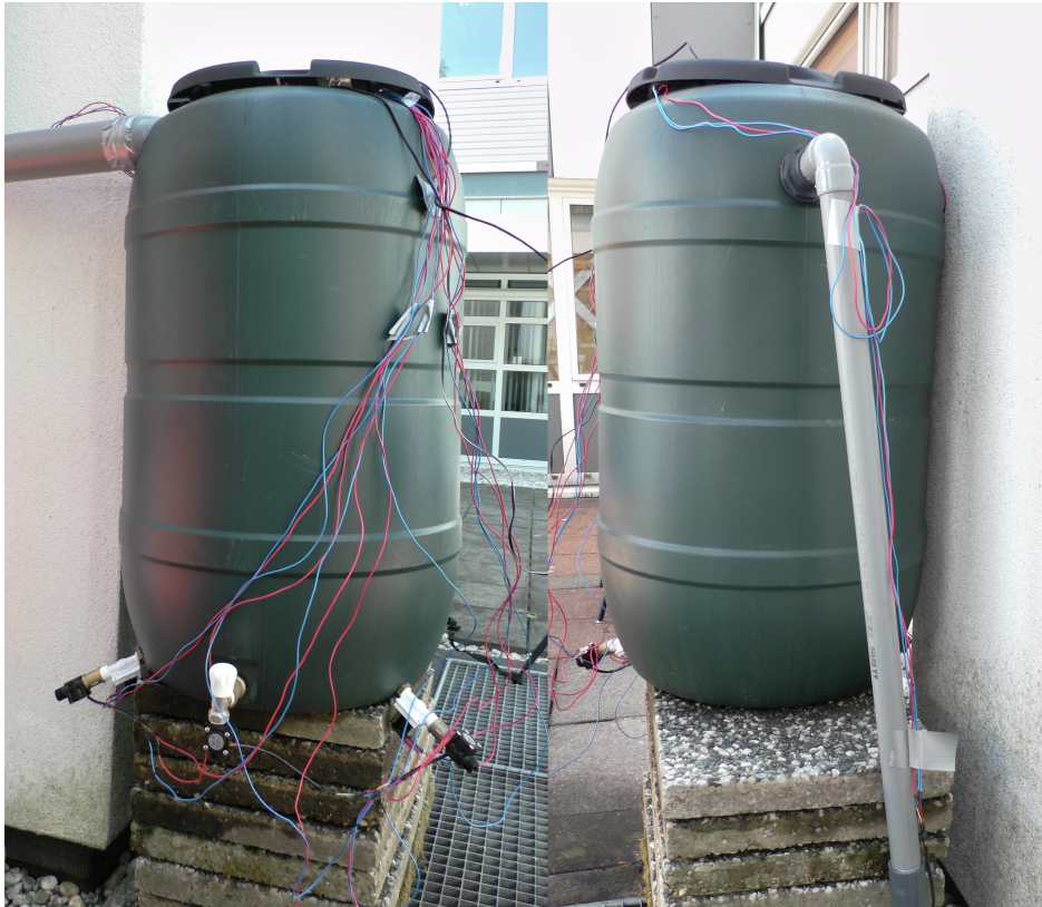
Figure 6.1: Left: the front of the barrel, with an input flow on the top and three output flows at the bottom. Right: the back of the barrel, with an overflow pipe to the sewers.
