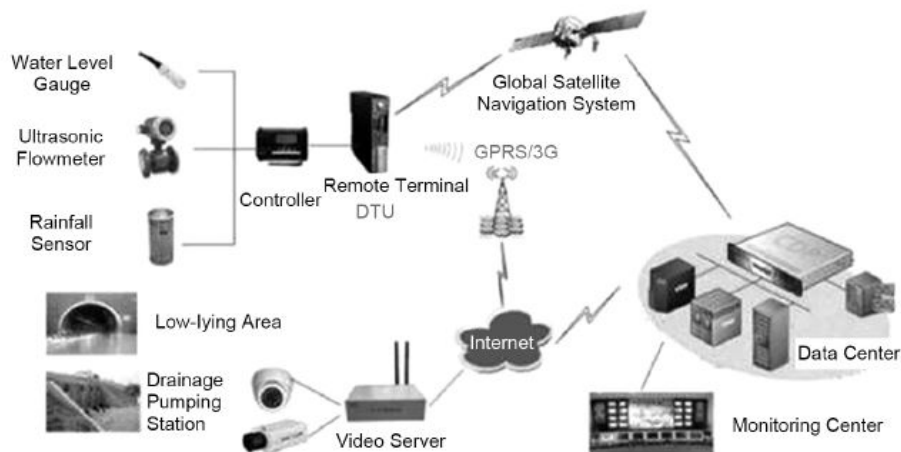
Figure 2.3: Internet of things applied to a monitoring system (Ma et al., 2017).
