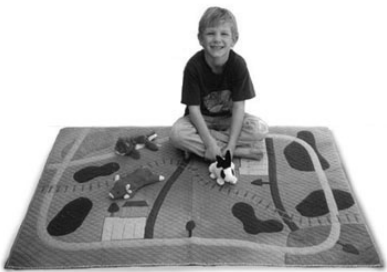
Figure 4.12 The StoryMat combines a physical map with sensor-integrated stuffed animals. Squeezing a stuffed animal triggers the recording of the movements of the animal and the sound created. Using similar coordinates as in a previous story triggers the beamer to show the previous story as a projection, MIT Media Lab , https://www.media.mit.edu/gnl/projects/storymat
