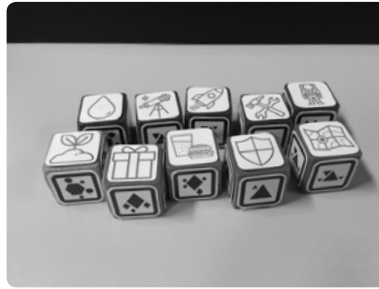
Figure 7.2 The prototype is extended with object blocks. The blocks have an icon on top and are equipped with markers to be recognised by the robot on the other sides.
