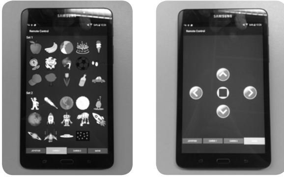
Figure 5.2 With the control tablet images can be selected to be used as story assets (left image), in addition, the tablet can be used to navigate the surfacebot in space (right image) by moving it [up and down arrow], rotating it clockwise and counter-clockwise [left and right arrow] and stopping it [central circle].
