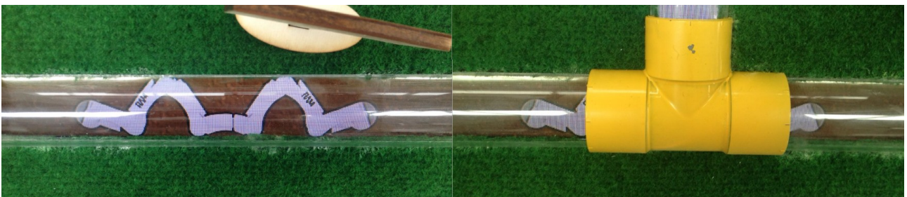
Figure 72: PIRATE picture version one inside pipe maze
