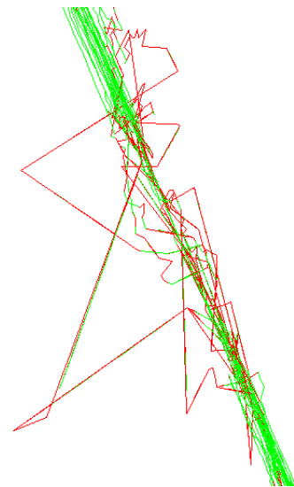
Figure 19: Recurring Signal Multipath Error ASPARi Archive: TWW Markelo 2016
