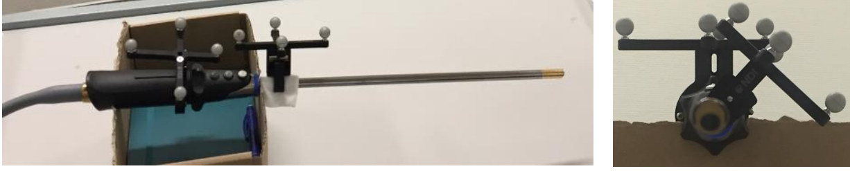
Figure 8: Top, side and front view of the Olympus EndoEye HD 10 mm with an oblique view angle of 30° and two optical frames attached for navigation.
