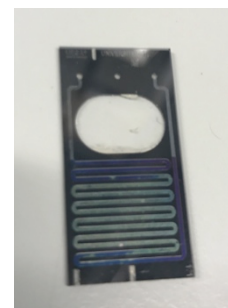
Figure 2.7 Picture of a chip wash coated with 20wt% \text{ZrO}_2 suspension.
