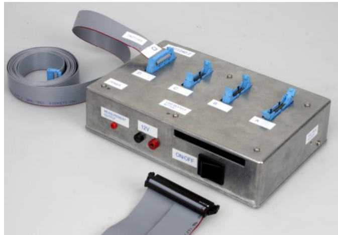
Figure 4. The amplifier with the 100-pin connector and the four 20 pin connectors labelled from A to D
