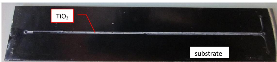
Figure 20. Patterned titania with 3 channels obtained with 30 wt% TiO<sub>2</sub> by using static method
