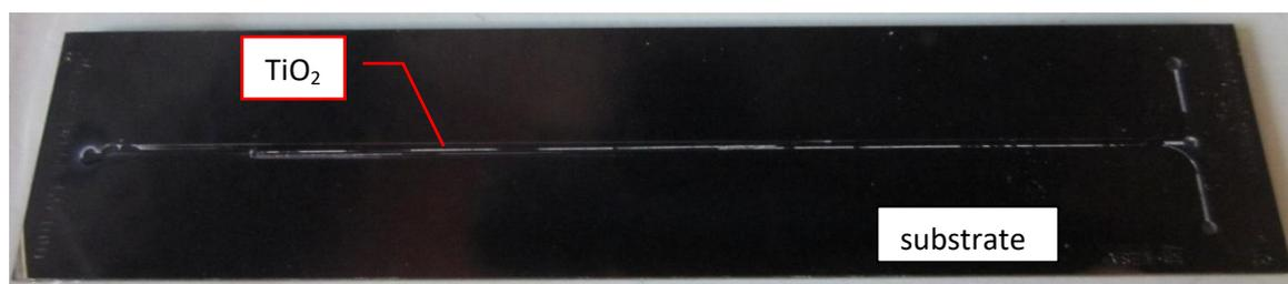
Figure 21. Patterned titania with 5 channels obtained with 30 wt% TiO<sub>2</sub> by using static method
