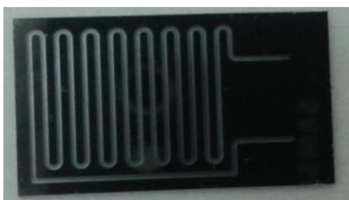
Figure 5. Microreactor with large channel (500  $\mu\text{m}$  width)
