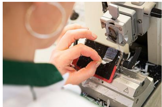
Figure 8 - Cutting a section of 0.002mm at the microtome (LabPON, 2017c)
