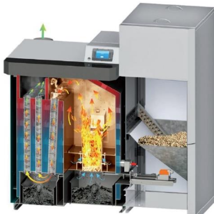
Figure 35 Profile section of a pallet stove system. [163]
