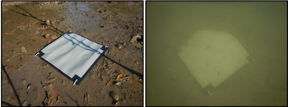
FIGURE 5. TESTING THE CANVAS SEDIMENT TRAP, FROM LEFT TO RIGHT: THE CANVAS TRAP DEPLOYED IN THE MANGROVE (A) AND THE BULGING EFFECT OF THE TRAP DURING HIGH TIDE (B).
