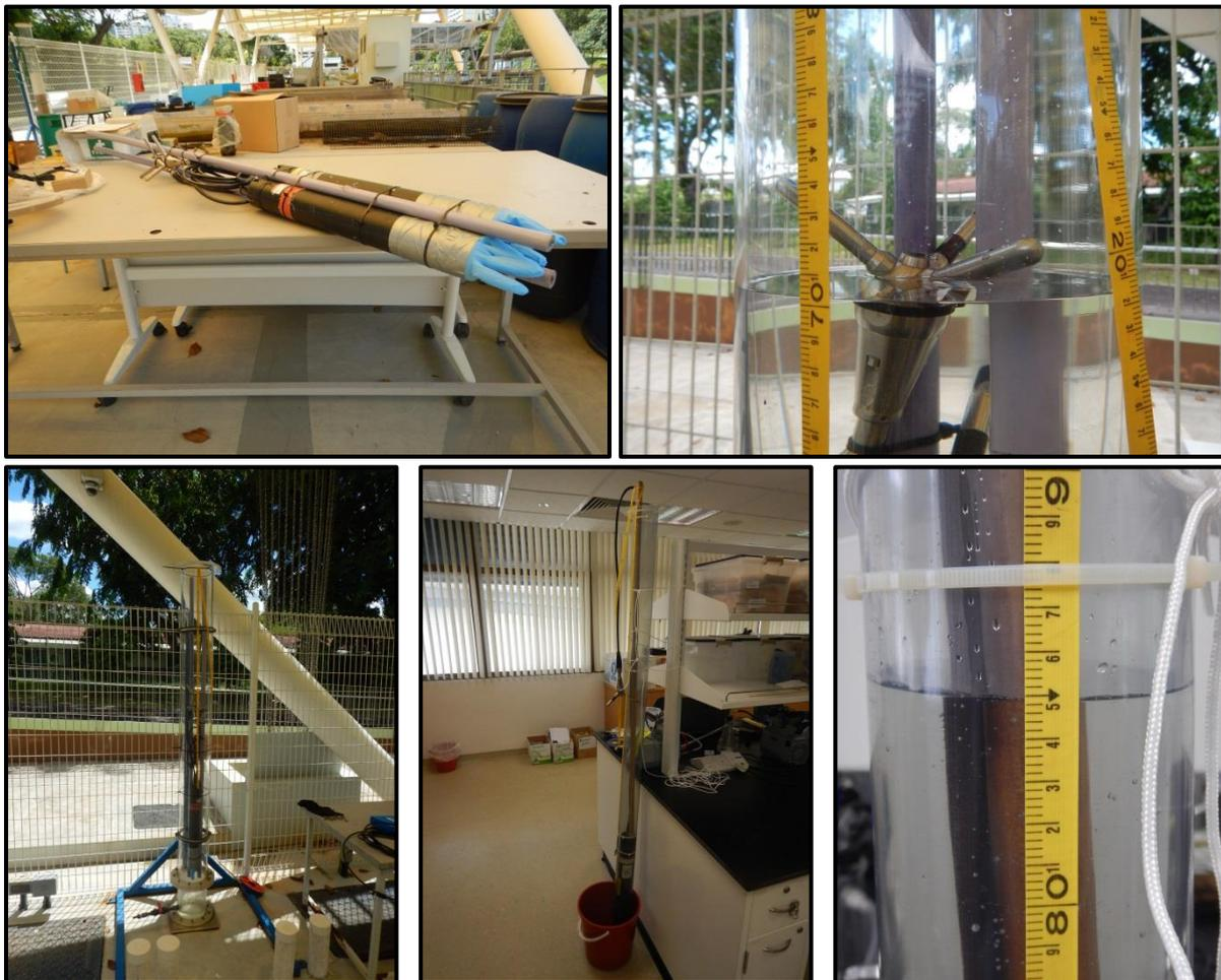
FIGURE 8. CALIBRATING THE PRESSURE SENSORS, FROM TOP LEFT TO BOTTOM RIGHT: MOUNTING ADV 1 (RED) AND ADV 3 (GREY) TOGETHER (A), MEASURING THE PRESSURE OF ADV 1 AND 3 AT A WATER LEVEL OF 0.7M (B), THE SET UP FOR MEASURING ADV 2 (BLUE) (D) AND MEASURING THE PRESSURE OF ADV 2 (BLUE) (E).
