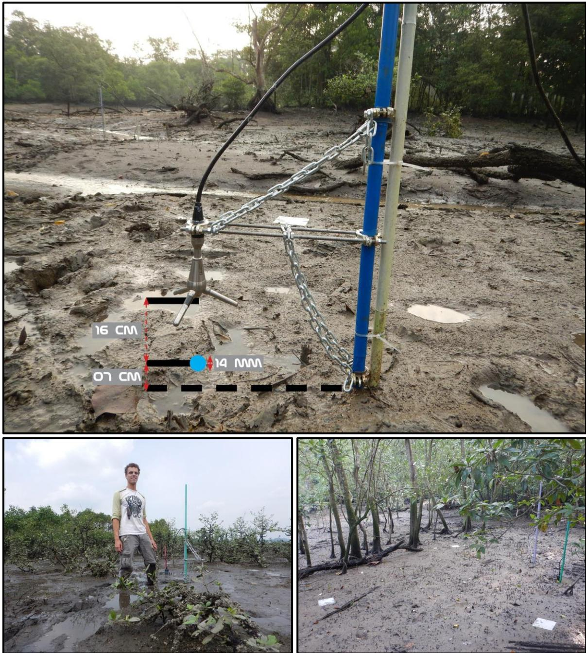
FIGURE 7. DEPLOYMENT OF THE ADVS, FROM TOP LEFT TO BOTTOM RIGHT: DIMENSIONS OF THE HEAD OF THE ADV, WITH THE MEASUREMENT VOLUME AS A BLUE DOT (A), DEPLOYED ADV AT THE *SONNERATIA* PATCH (B), DEPLOYED ADV AT THE BACK OF THE MANGROVE (C).
