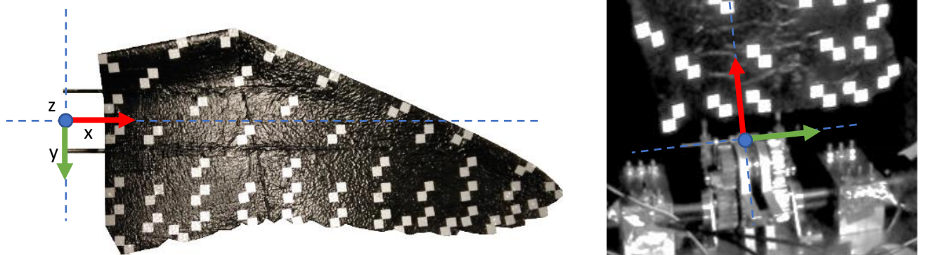
Figure 3: Left: Wing reference frame O_{wing} with origin at pivot point, indicated on an older version of the wing. Right: Cropped video frame showing the pivot point.
