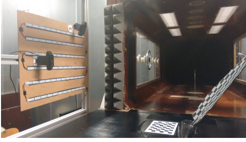
Fig. 5. The imaging setup in the wind tunnel (left) includes an LED stroboscope driven by an Arduino Uno, and two webcams that are read out simultaneously.
