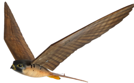
Fig. 1. The Robird: peregrine falcon model.
