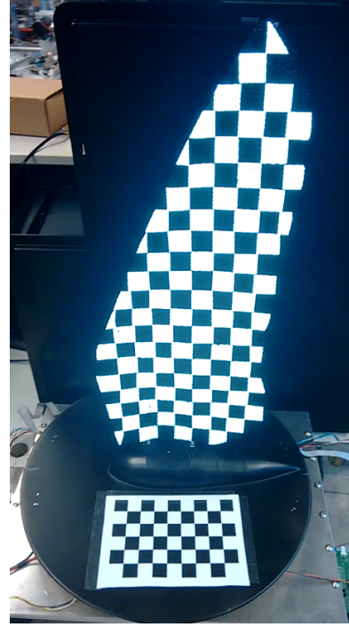
Fig. 6. The wing is covered in black spray paint and a checkerboard pattern made of reflective tape. This increases contrast, and provides many keypoints for tracking. It also allows to apply 2D strip kinematics to the wing. An additional static checkerboard on the windshield defines a world reference frame.
