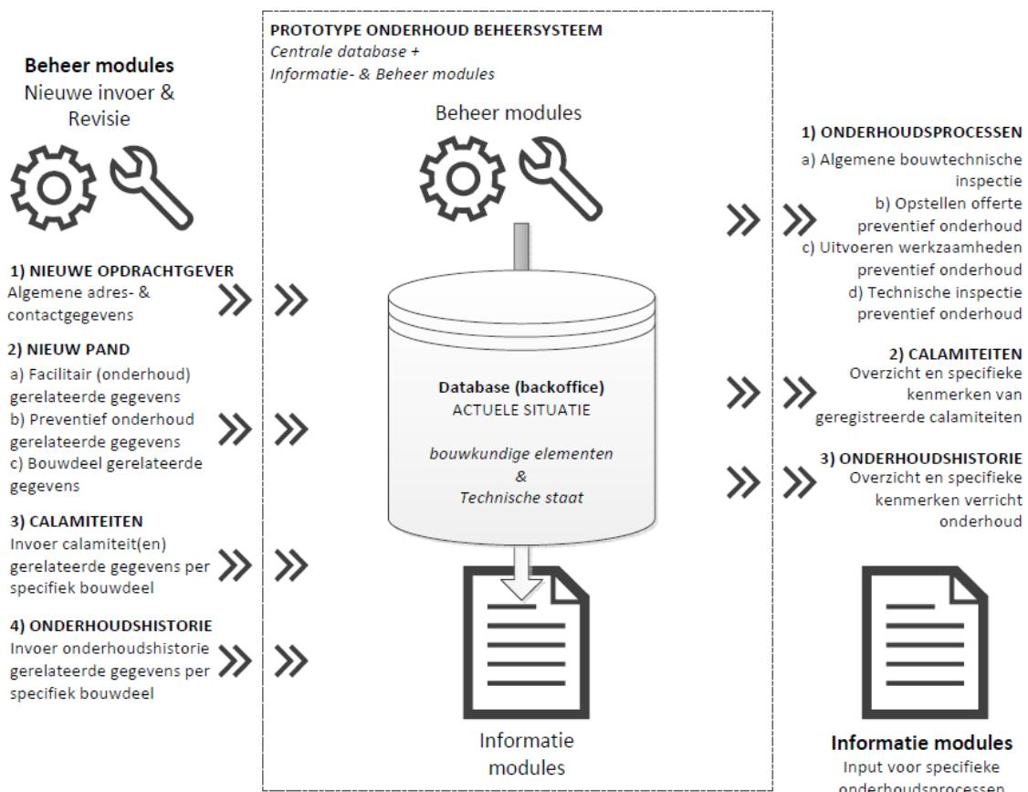
Figure 14: Functionality of prototype information system
