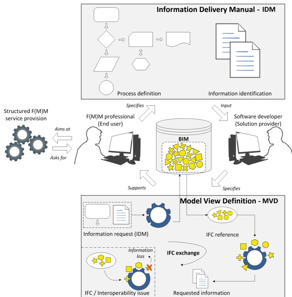
Figure 3: Gap analysis – IDM and MVD developments to support F(M)M service provision
