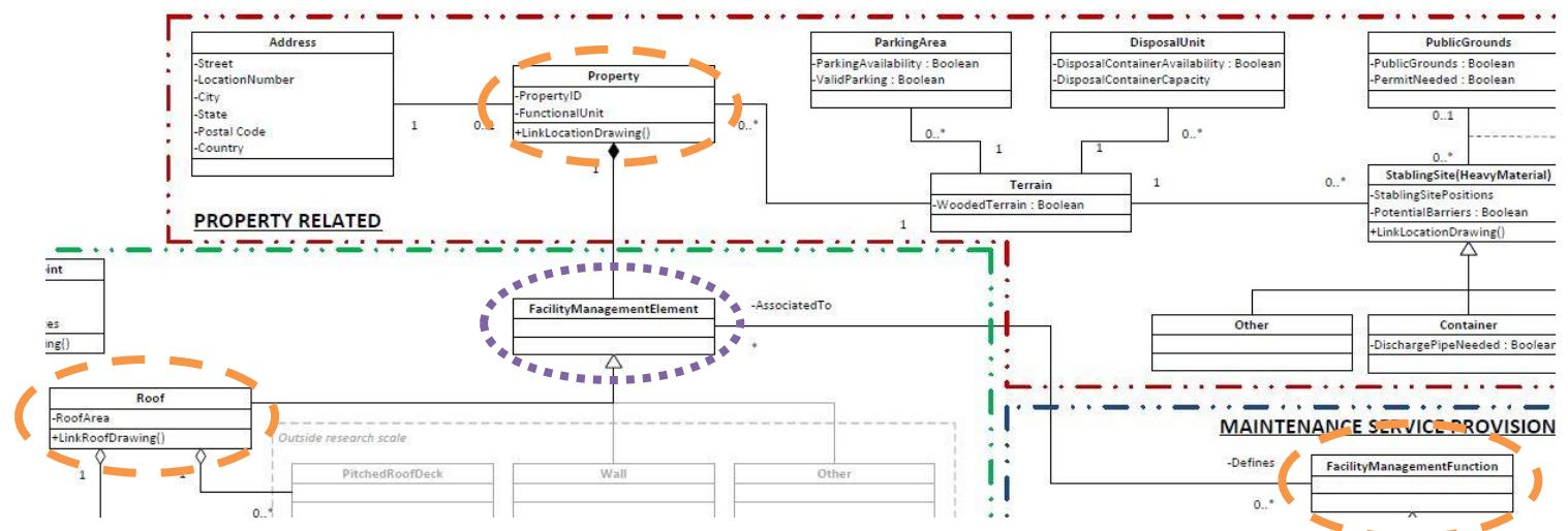
Figure 12: Core (top-classes) of the class model
