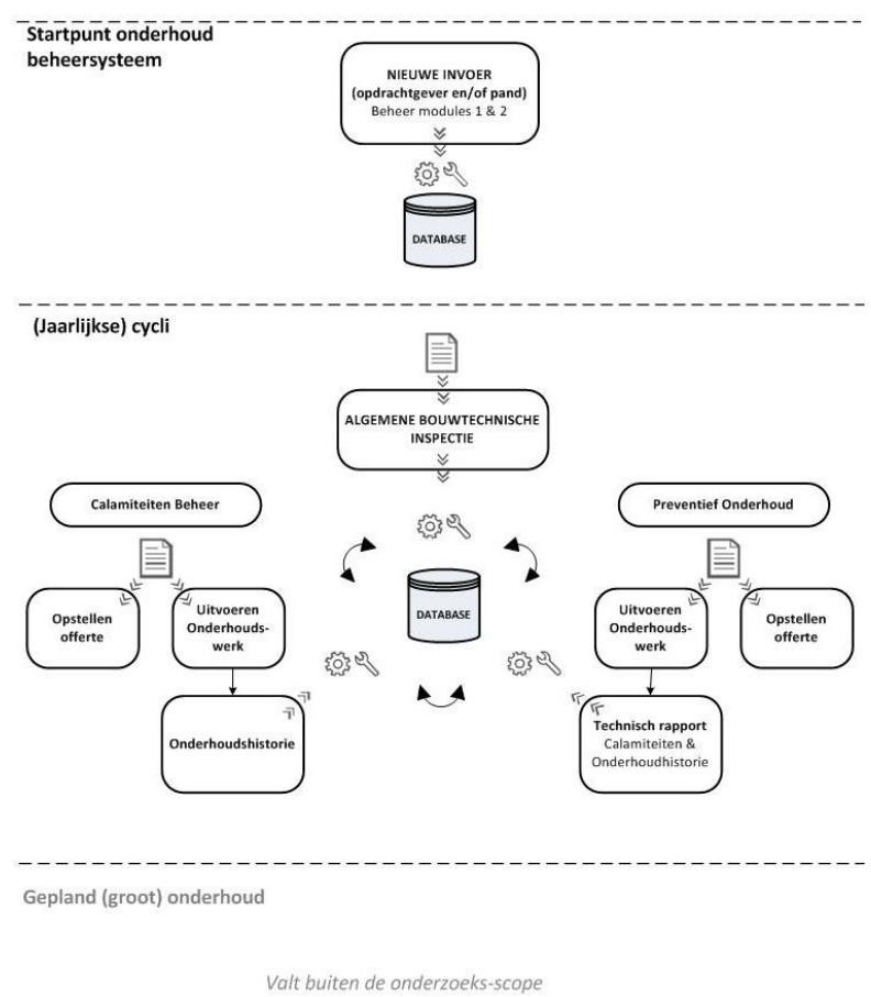
Figure 11: Use Case integration regarding desired information system in relation to the improved annual maintenance cycle and defined information modules
