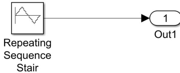
(c) Triangular wave generator (carrier)
