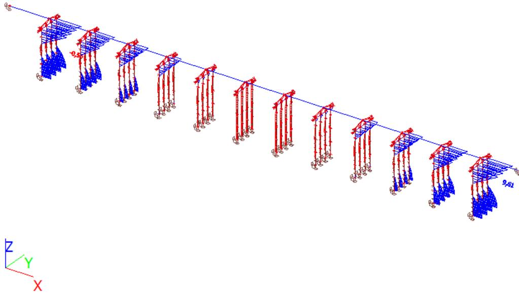
Figure 52 Resulting stress on the poles with the ULS loads
