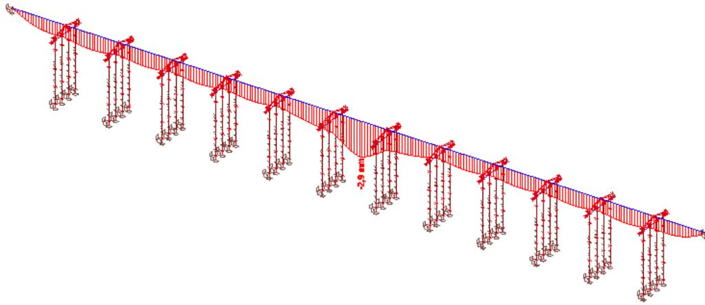
Figure 54 Resulting displacement on the tunnel cross section with sunken vessel loads
