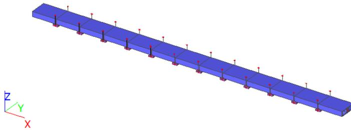
Figure 39 Overview of the pontoon submerged floating tunnel design
