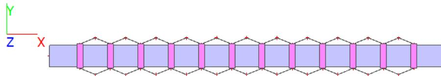
Figure 49 View from above the tethered type of submerged floating tunnel design
