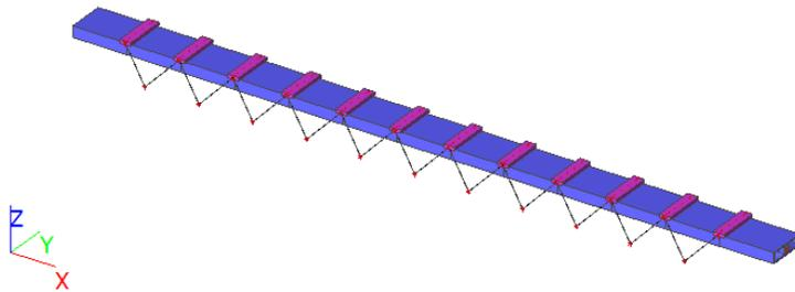
Figure 47 Overview of the tethered type of submerged floating tunnel design
