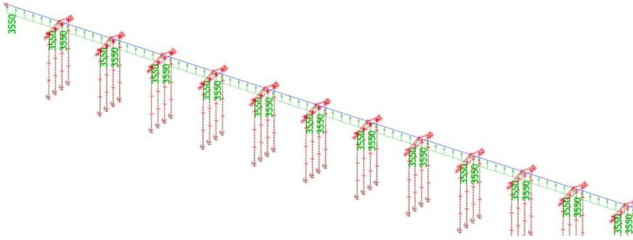
Figure 10 the load created by the buoyancy modelled on the pressure-bearing-poles SFT reference design
