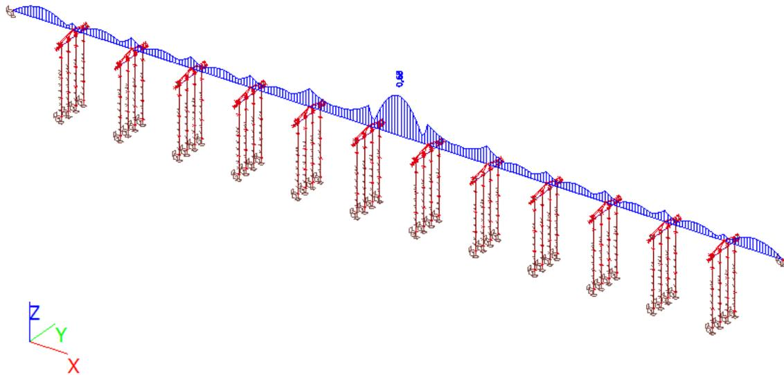
Figure 62 Resulting stress on the tunnel cross section with partially flooded loads
