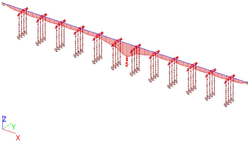
Figure 63 Resulting displacement on the tunnel cross section with partially flooded loads
