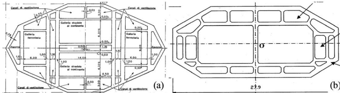
Figure 3 rectangular tunnel with triangular steel frame (a) and rectangular tunnel with smoothed edges (b) (Martire, 2010)
