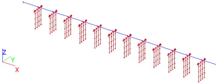
Figure 42 Overview of the submerged floating tunnel with pressure-bearing-poles model
