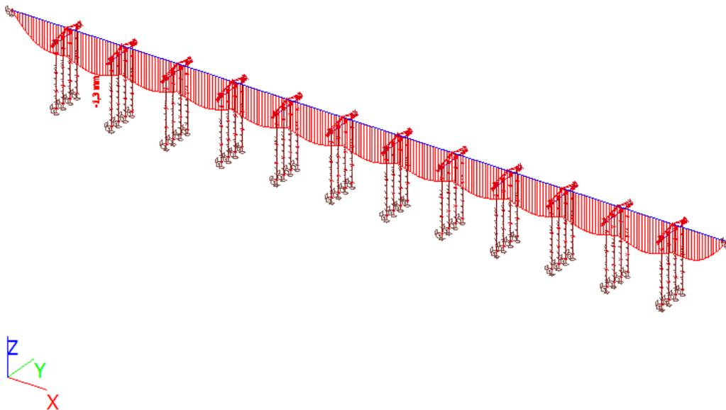
Figure 57 Resulting displacement on the tunnel cross section with tsunami loads
