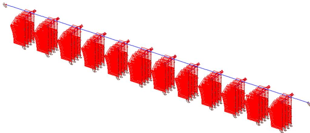
Figure 55 Resulting stress on the poles with the sunken vessel loads
