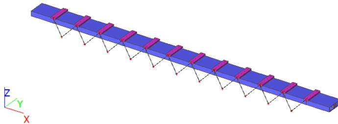
Figure 26 the tethered type of SFT reference design
