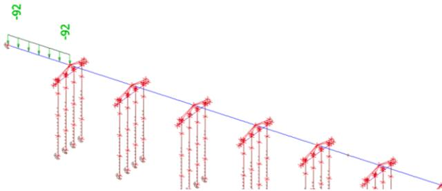
Figure 13 the load created by the traffic modelled on the pressure-bearing-poles SFT reference design
