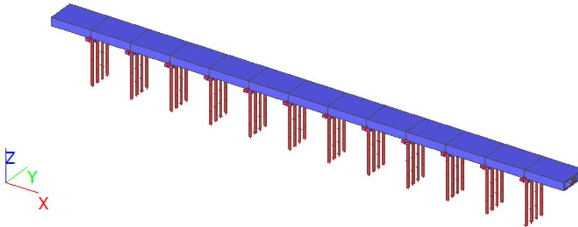
Figure 43 Overview of the submerged floating tunnel with pressure-bearing-poles design
