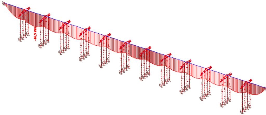
Figure 60 Resulting displacement on the tunnel cross section with fully flooded loads
