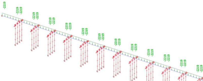
Figure 16 the load created by total flooding modelled on the pressure-bearing-poles SFT reference design
