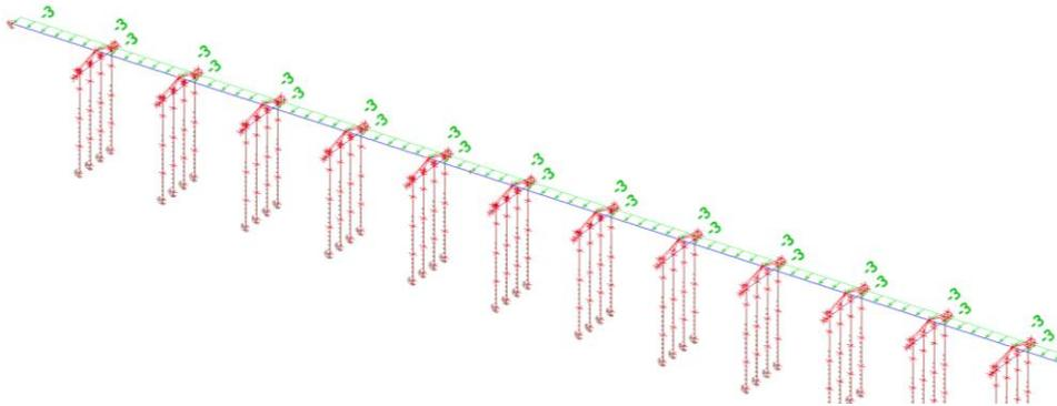
Figure 14 the load created by the current modelled on the pressure-bearing-poles SFT reference design
