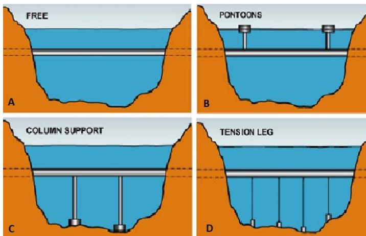
Figure 1 the four types of submerged floating tunnels (Mohan, 2011)
