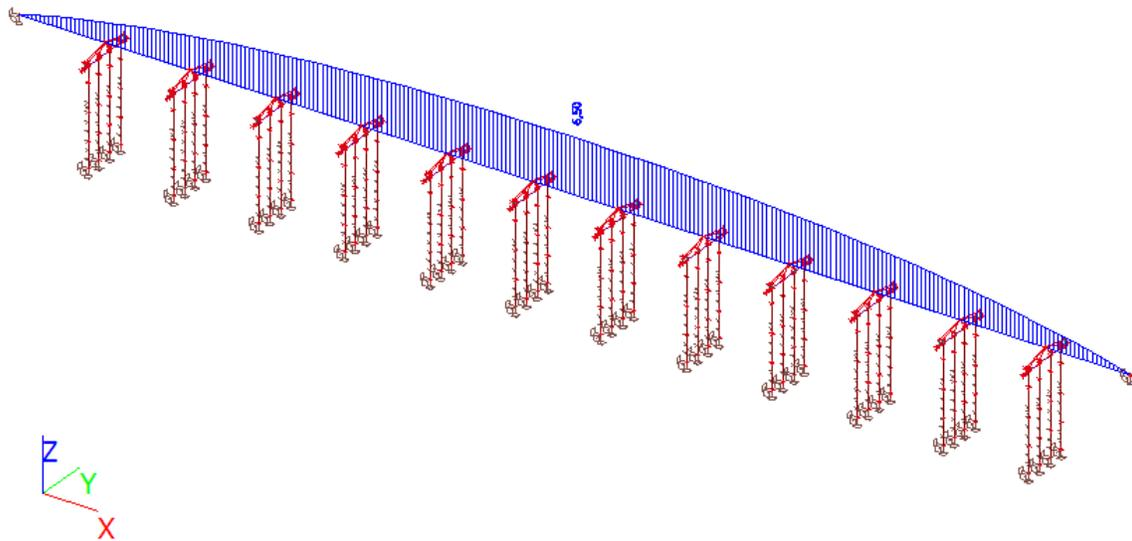
Figure 56 Resulting stress on the tunnel cross section with tsunami loads
