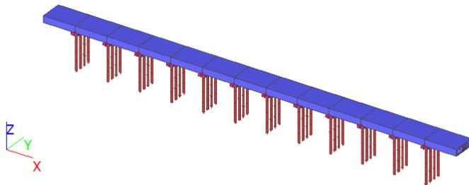
Figure 25 the SFT with pressure-bearing-poles reference design
