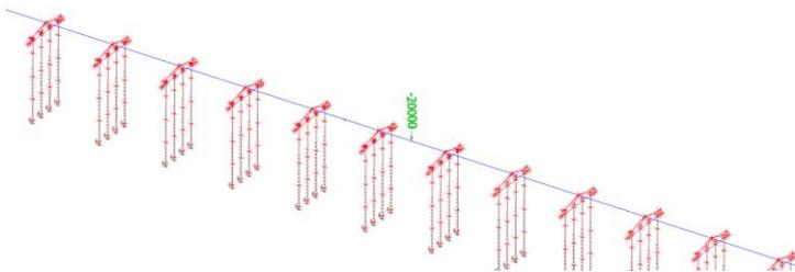
Figure 19 the load created by a sunken vessel modelled on the pressure-bearing-poles SFT reference design
