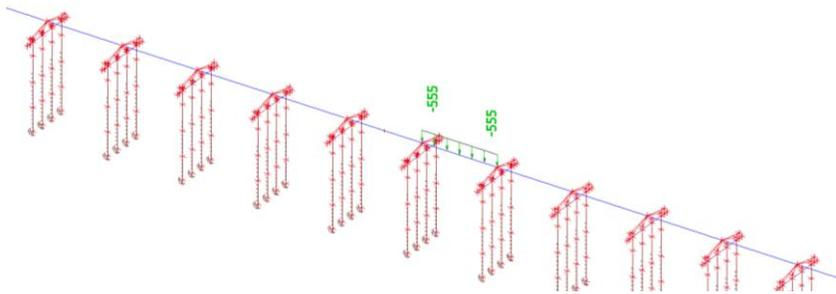
Figure 17 the load created by partial flooding modelled on the pressure-bearing-poles SFT reference design
