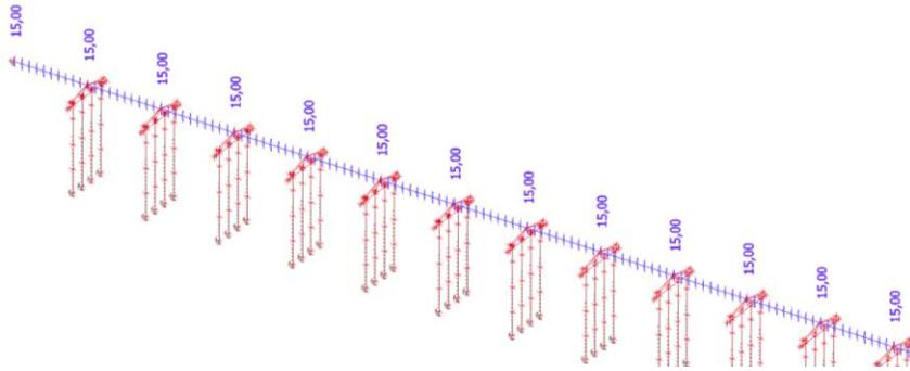
Figure 15 the thermal load modelled on the pressure-bearing-poles SFT reference design
