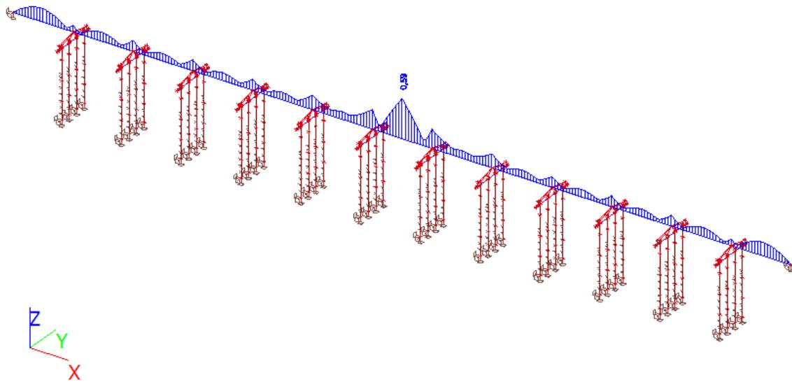
Figure 53 Resulting stress on the tunnel cross section with sunken vessel loads
