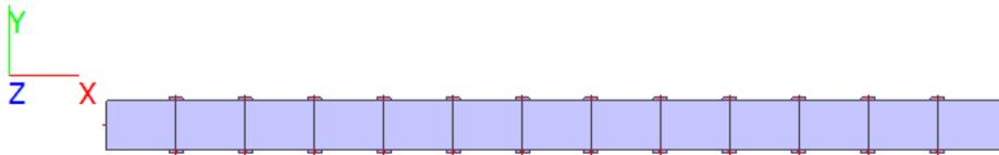
Figure 45 View from above of the submerged floating tunnel with pressure-bearing-poles design
