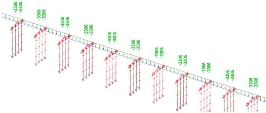
Figure 9 the load created by the self-weight modelled on the pressure-bearing-poles SFT reference design
