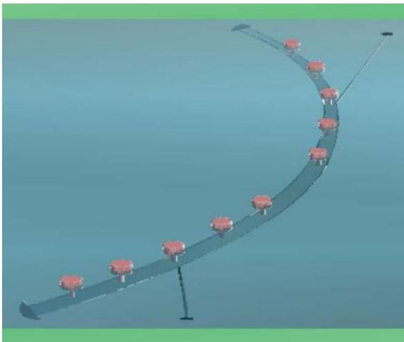
Figure 28 an example of an arced pontoon SFT (Jakobsen, 2010)
