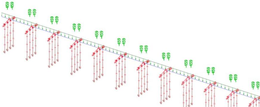
Figure 11 the load created by the ballast concrete modelled on the pressure-bearing-poles SFT reference design
