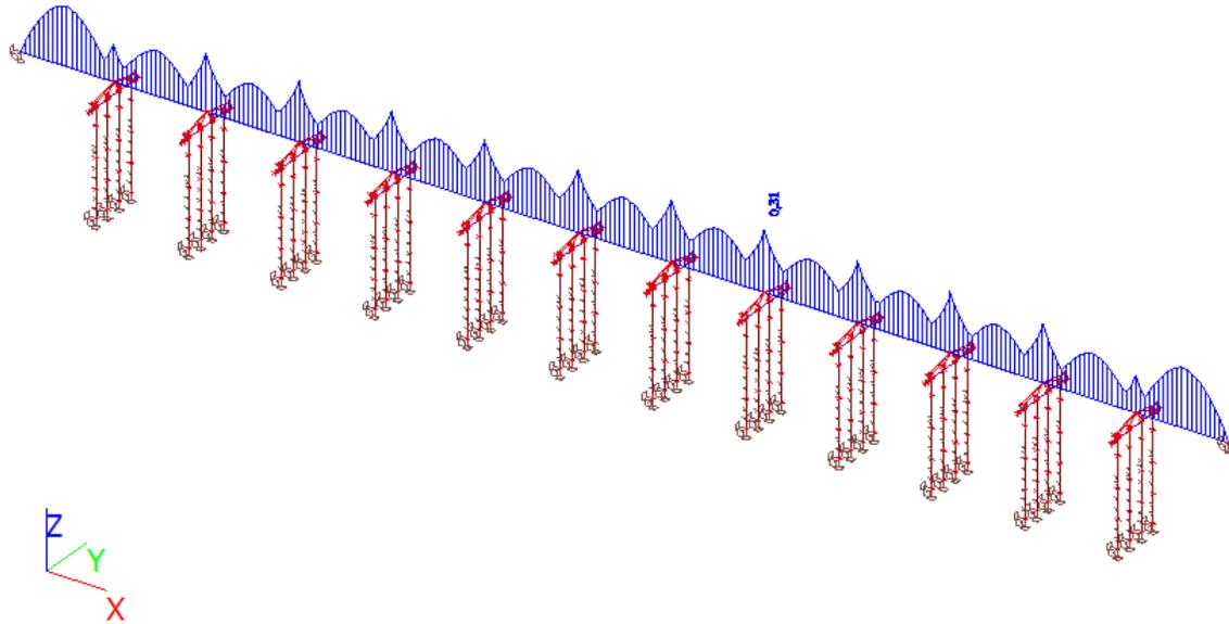
Figure 50 Resulting stress on the tunnel cross section with ULS loads
