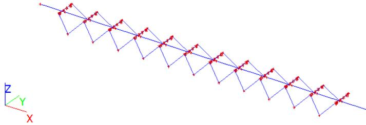
Figure 46 Overview of the tethered type of submerged floating tunnel model
