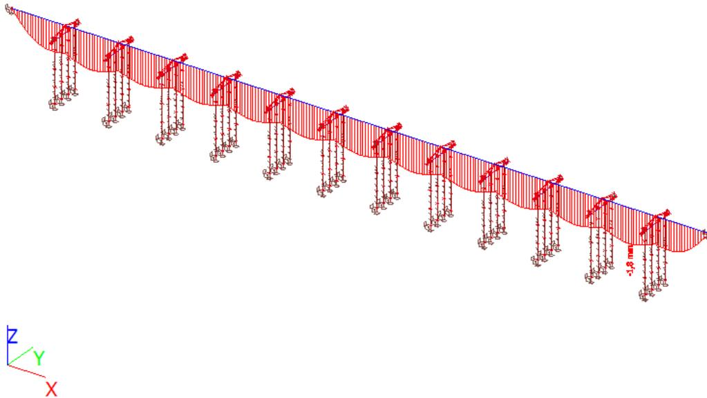
Figure 51 Resulting displacement on the cross section with ULS loads
