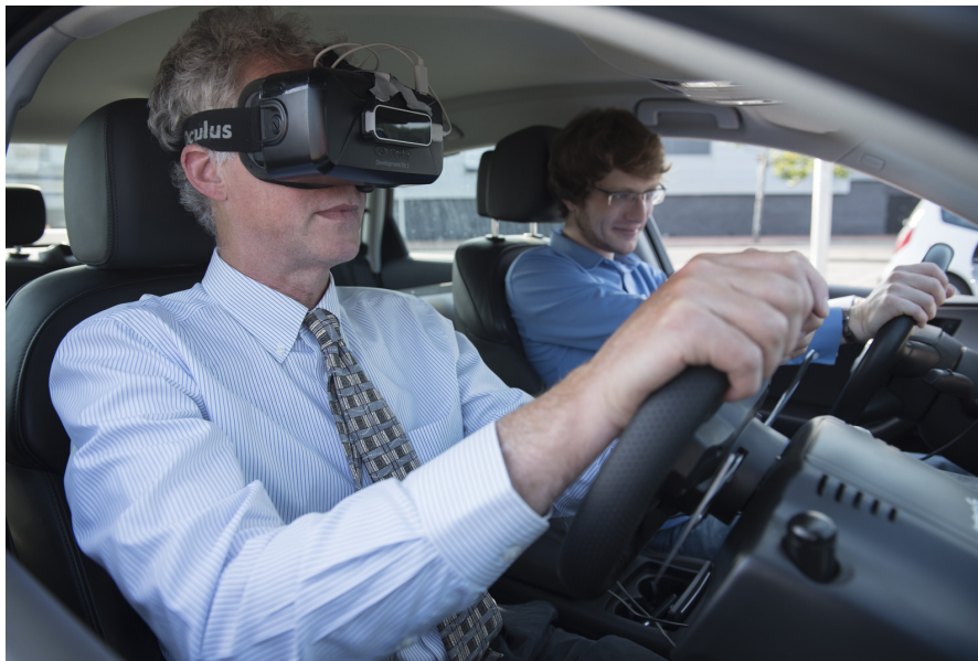
Figure 1.1: VR-in-Car allows participants to experience the physical sensations of real-world motion while being visually in a virtual environment.
