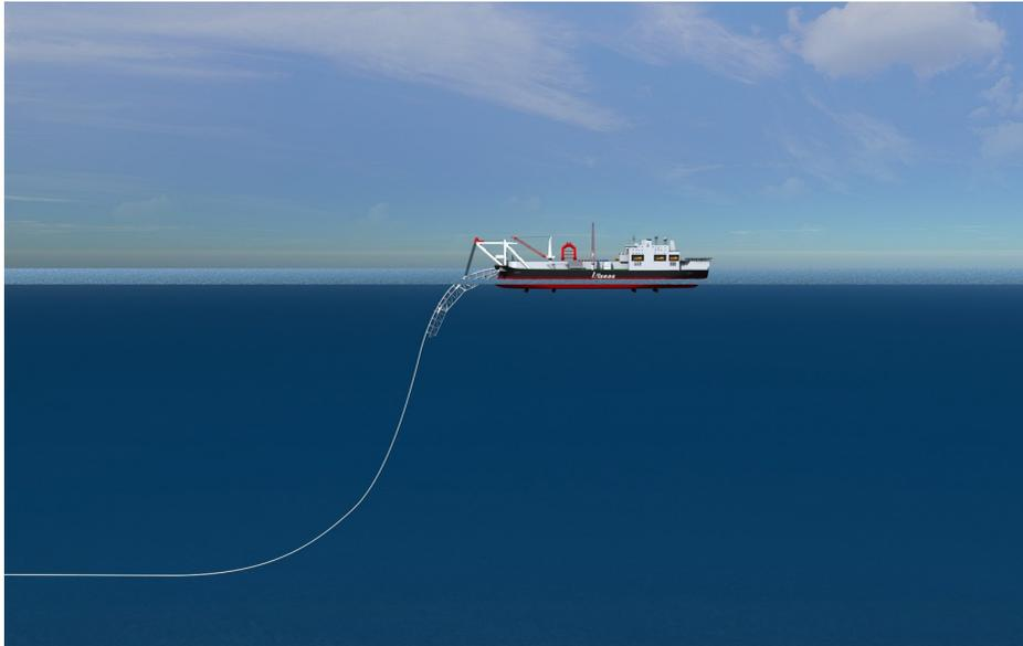
FIGURE 1.1: The S-lay method performed by an Allseas ship. The pipe is produced and released from the back-end of the ship, supported by the stinger. It goes downwards until it reaches the already laid pipe supported by the seabed.
