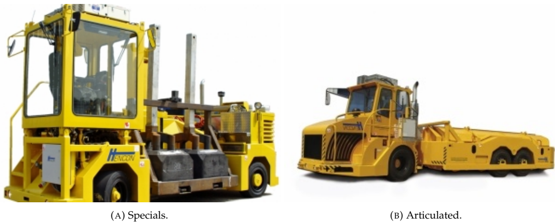
FIGURE 1.4: Examples of anode pallet transport vehicles
