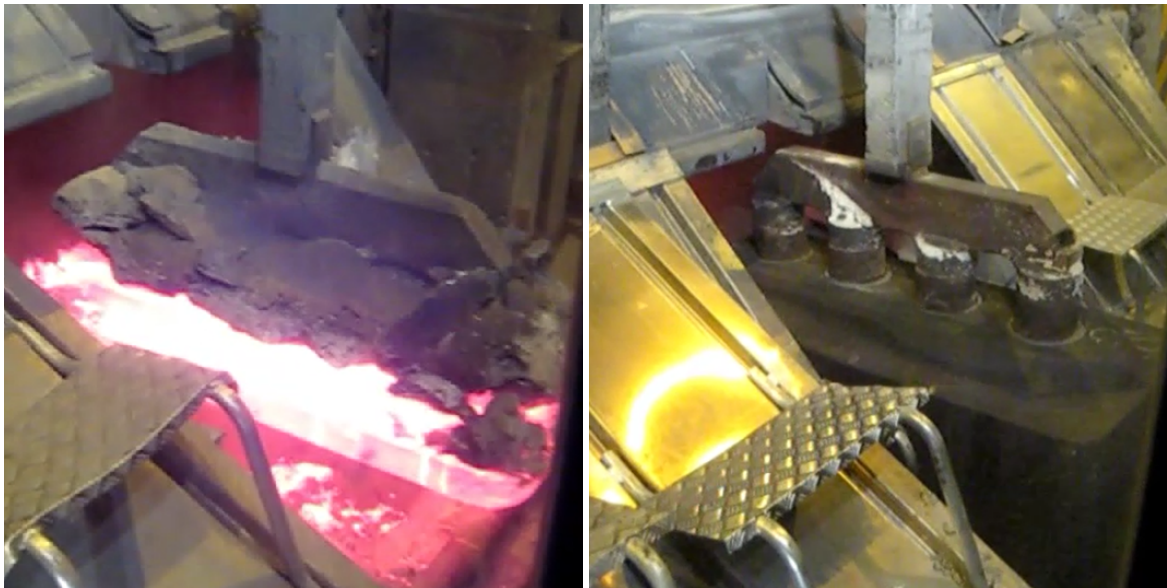
(A) Anode taking. A burned anode is removed from an (B) Anode placing. An fresh anode is placed in an electrolytic-cell.
