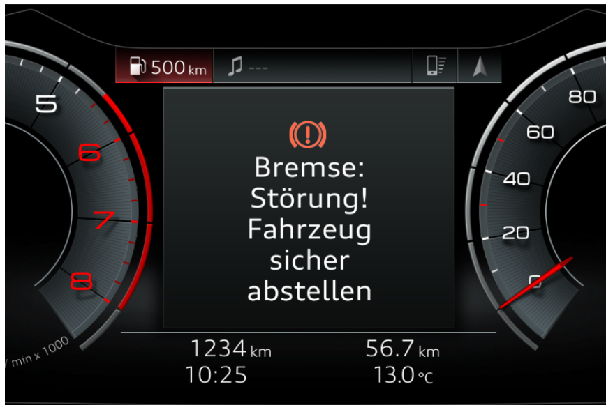
Figure 7. Screenshot of the Audi digital car instruments with the warning ‘Break: Error! Stop car safely’.
