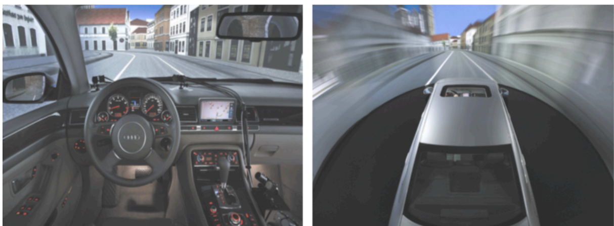
Figure 3. Interior ( left ) and exterior ( right ) of the driving simulator.
