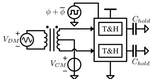
Figure 6.7: Testbench for track and hold linearity simulation in *Spectre/Cadence*.
