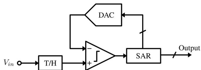
Figure 1.2: Block diagram of a single-ended SAR ADC.
