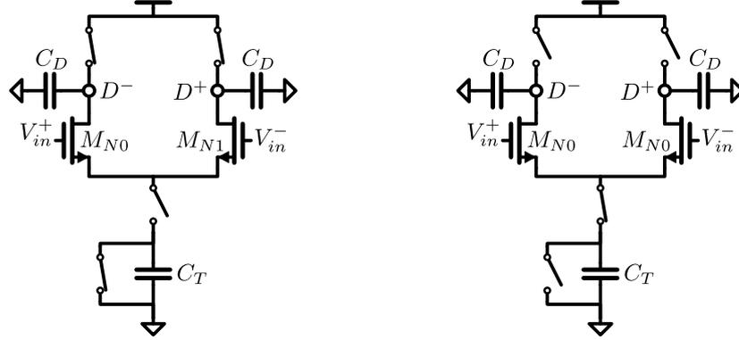
Figure 4.2: Pre-amplifier: Left: Reset-phase. Right: Comparison-phase.
