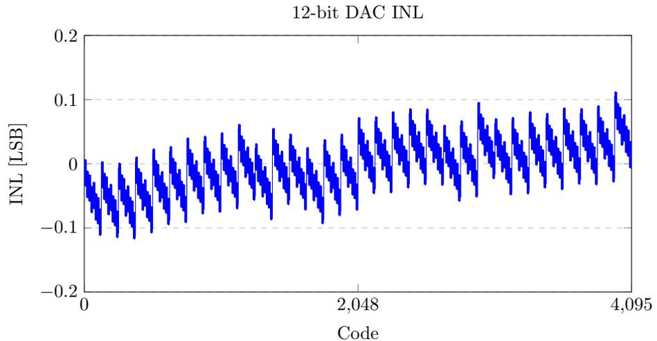
Figure 6.3: DAC INL simulation result.
