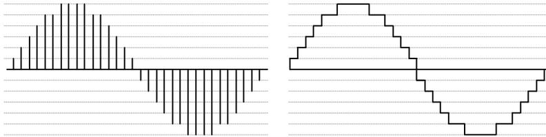
Figure 1.4: Graphical representation of digital-to-analog conversion.
