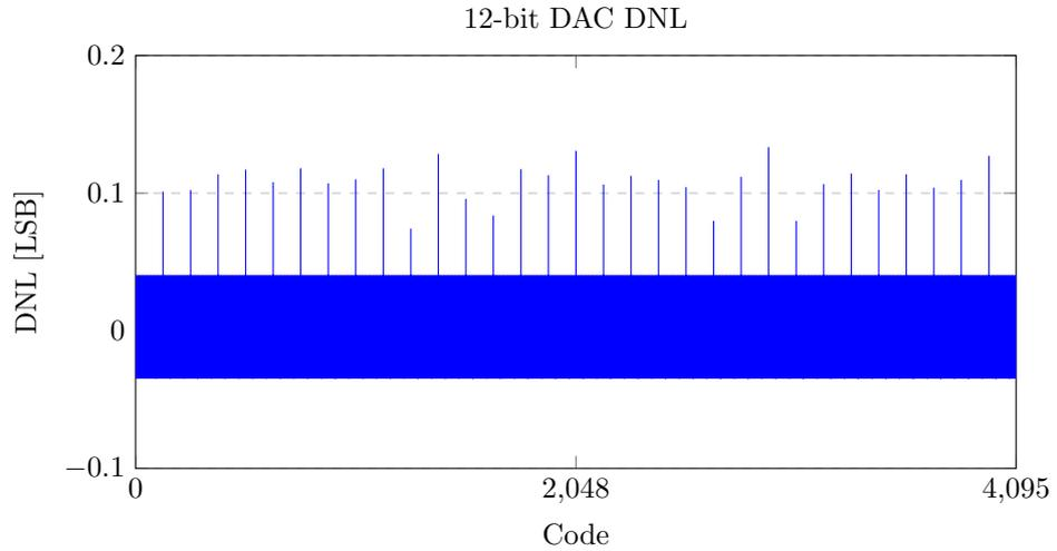
Figure 6.2: DAC DNL simulation result.
