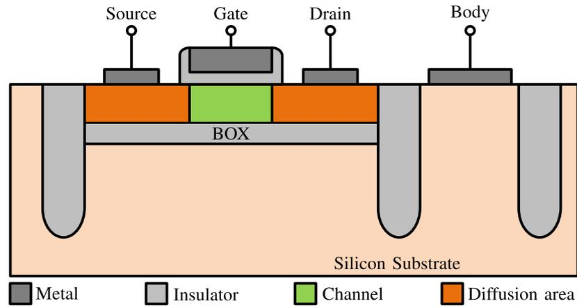
Figure 1.6: FD-SOI MOSFET structure.
