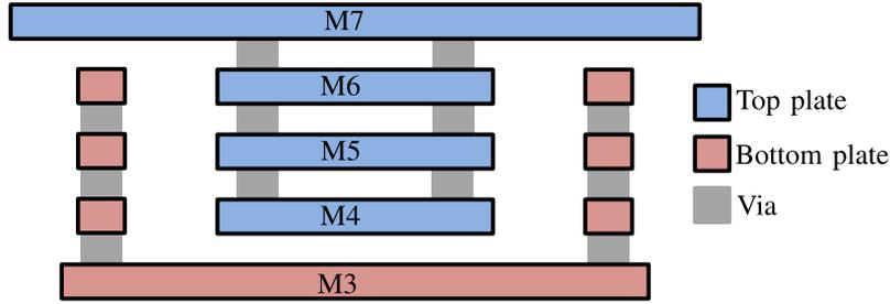
Figure 3.4: Cross-sectional view of proposed MOM capacitor.
