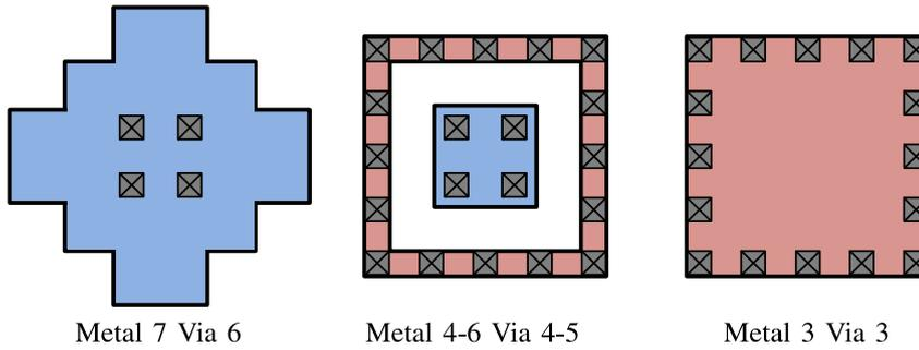
Figure 3.5: Top view of proposed MOM capacitor.
