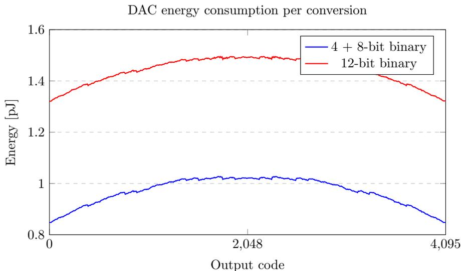
Figure 6.4: DAC energy simulation result.
