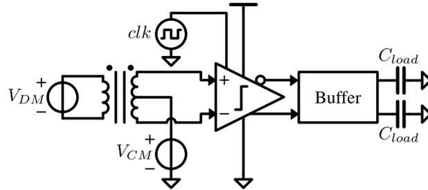
Figure 6.5: Testbench for comparator simulation in *Spectre/Cadence*.
