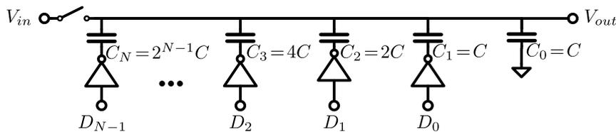
Figure 1.5: Capacitive charge-redistribution DAC.
