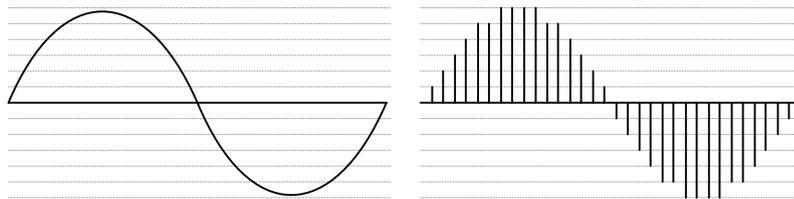
Figure 1.1: Graphical representation of analog-to-digital conversion.
