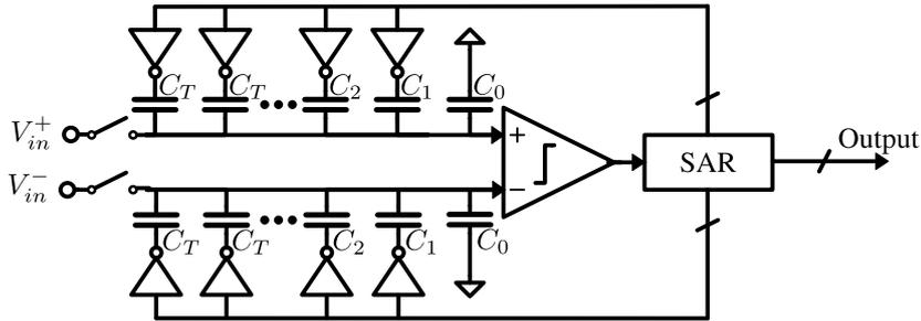
Figure 3.1: Block diagram of a differential partially thermometer-coded SAR ADC.
