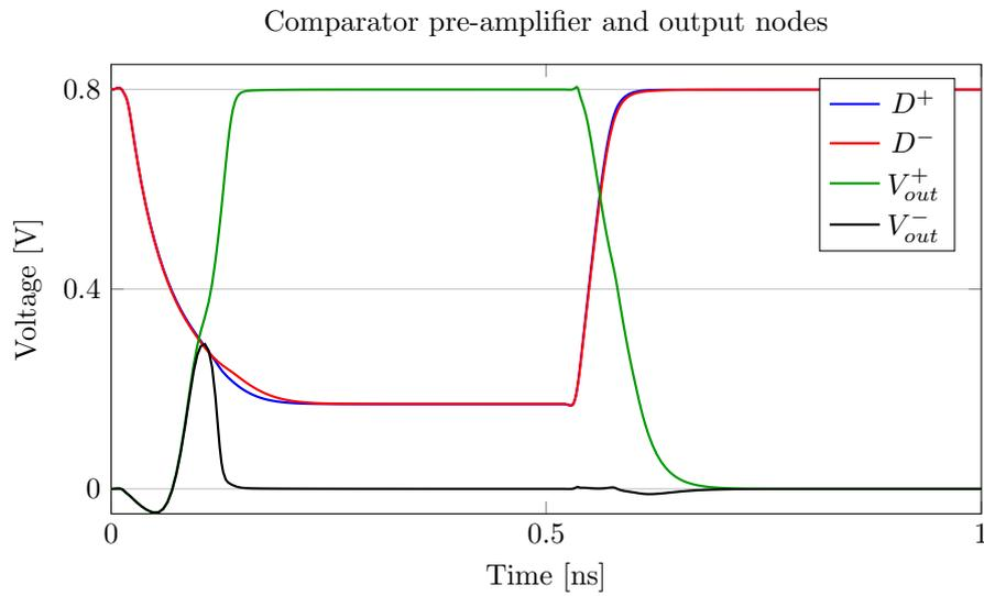
Figure 6.6: Pre-amplifier and output signals for  $V_{DM} = 300\mu V$ .
