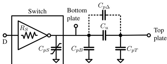
Figure 3.2: (MOM) unit capacitor model.
