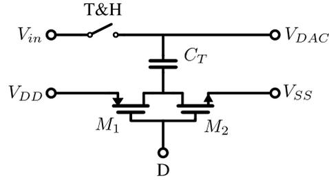
Figure 3.7: DAC capacitor inverter switch.
