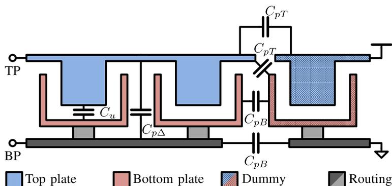
Figure 3.3: cross section of the DAC showing parasitics.
