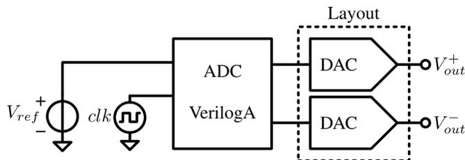
Figure 6.1: Testbench for the DAC linearity simulation in *Spectre/Cadence*.
