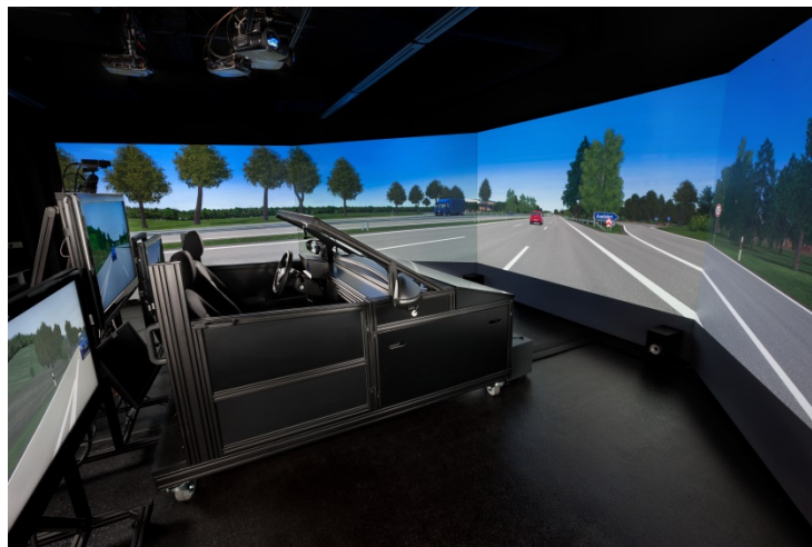
Figure 11. The fixed-base lab demonstrator in front of three 4x4m canvases. The two canvases at the very left and the very right have not been used in this study. Three additional mounted screens allowed the participant to take a look in the rear and side mirrors.
