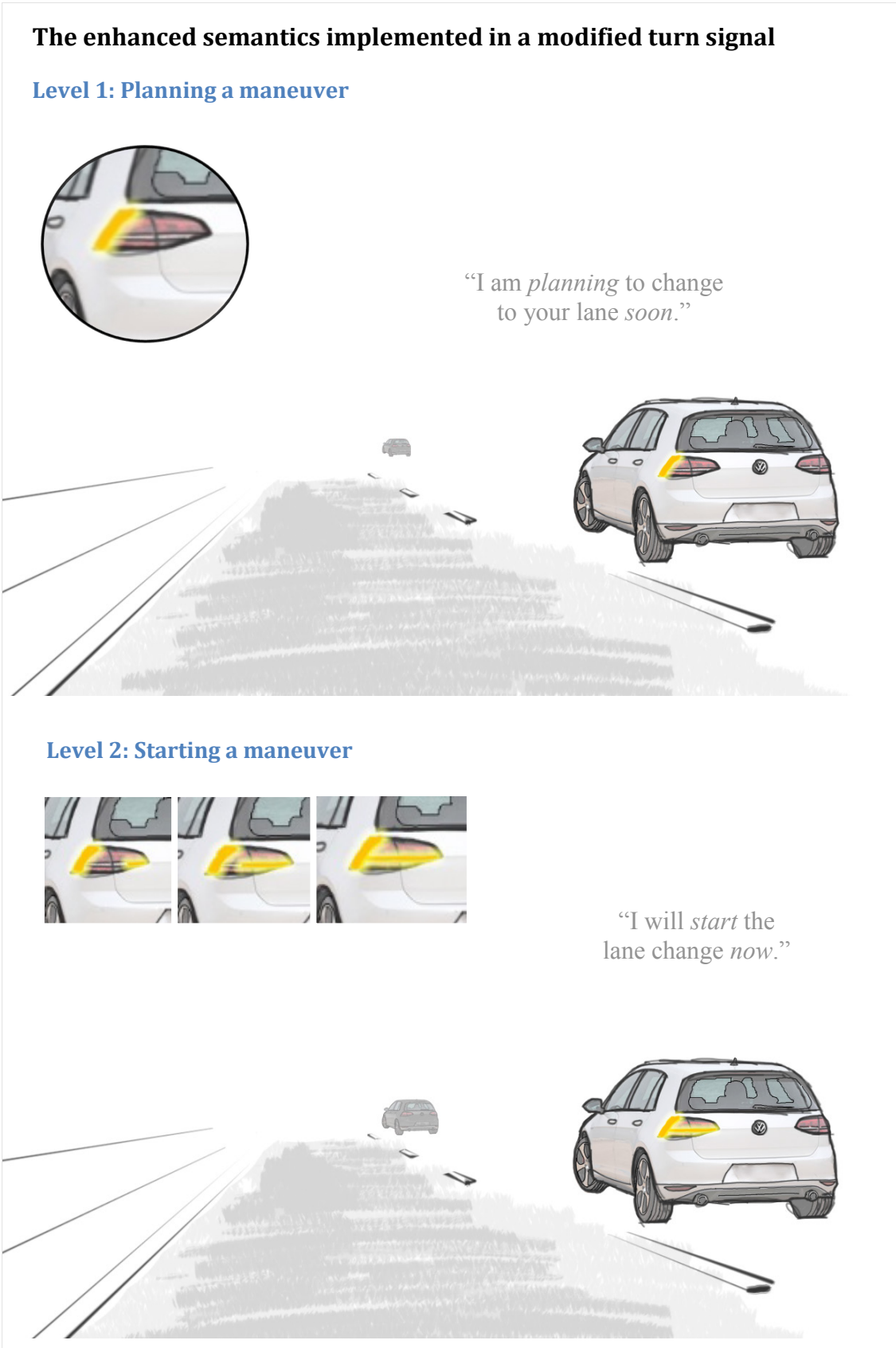
Figure 6. This figure shows the final version of the modified turn signal which resulted from the prestudy. It shows how the enhanced semantics are visualized in a modified turn signal.
