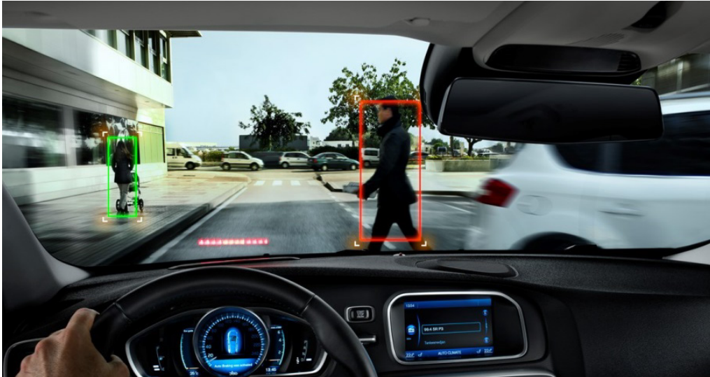
Figure 4. Volvo's concept of an augmented reality head-up display. A pedestrian is marked with a red outline to draw the driver's attention towards him (Volvo, 2014)
