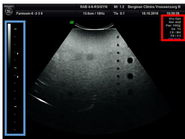
Figure 3, image made with Bergman device. The settings are visible in the red box. The focus is visible in the blue box.
