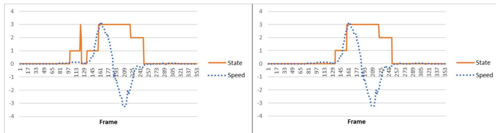
Figure 7.19 Left: example of noisy state prediction (HMM II) in exercise 8 executed by participant 3 on the right the corrected version.
