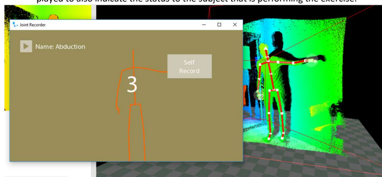
Figure A.3 While testing various exercises, a self-recording functionality is added. With your wrist, you can hit the self-record button when after this a count down appears. After this count down the recording starts. When finishing the recording the last second of data is removed as this only corresponds to raising the arm to the button again.
