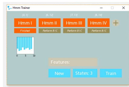
Figure 7.10 Application to train HMMs and quickly analyse BIC scores to determine states required during training
