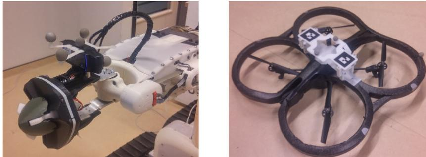
(a) OptiTrack markers placed on the camera - (b) OptiTrack markers placed on a AR Parrot 2.0 Drone and gripper interface
