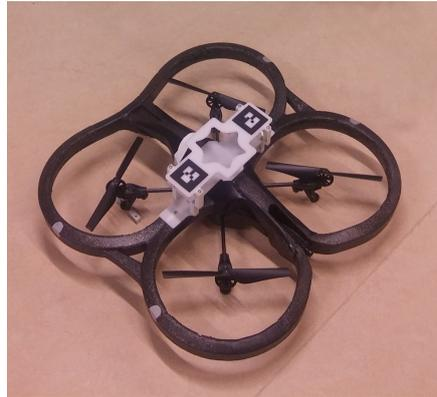
**Figure 5.2:** AR Parrot 2.0 Drone equipped with markers and gripper interface
