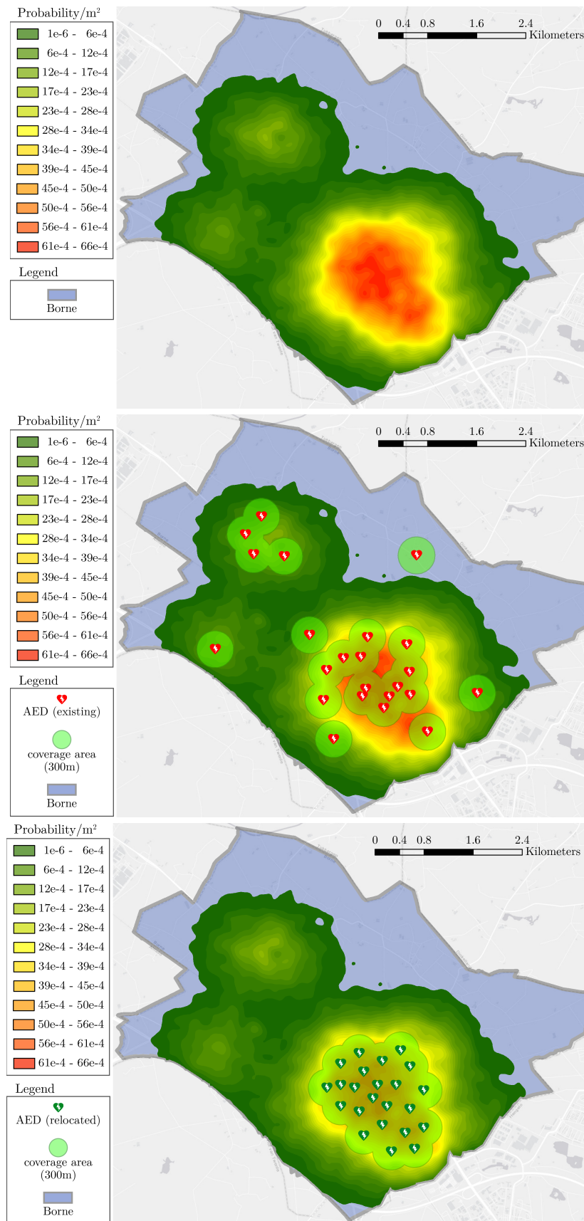
Figure 5.5: Locations of 23 AEDs in the municipality of Borne. Top image: cardiac risk probability distribution (KDE method); center image: current deployment of existing AEDs (8.2% coverage); bottom image: optimized deployment by relocating existing AEDs (11.5% coverage).
