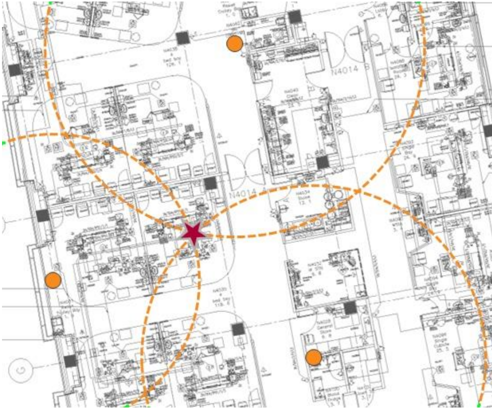
Appendix F: Triangulation to determine the location of a tag
