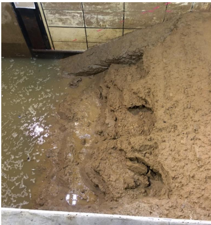
Figure 9 dike after 1,5 hour of testing waterboard I
