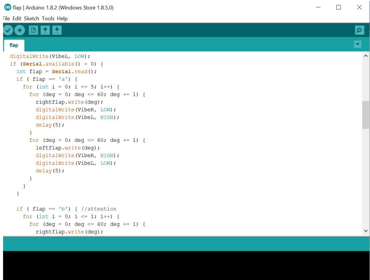
Figure 17: Arduino IDE with sample code for flap operation
