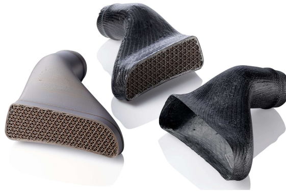
Figure 9 – Sacrificial composite tooling: Left – tool, middle – tool with part, right – resulting part.
