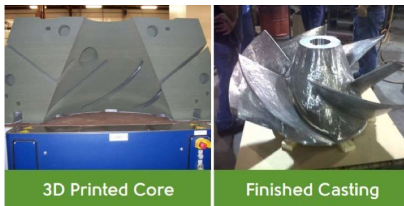
Figure 6 – 3D printed sand casting core and casted result (Maxey, 2015)
