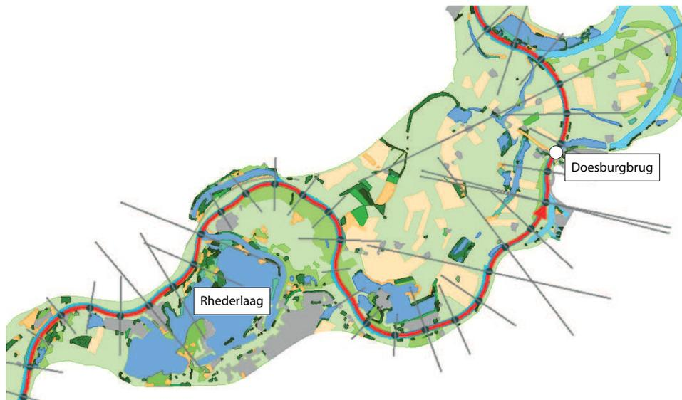
Figure 3.5: 1D schematization of the IJssel bend at the Rhederlaag near Doesburgbrug compared to the actual floodplain width. Red line indicates main channel, grey lines perpendicular to main channel indicate size of 1D cross-sectional profiles
