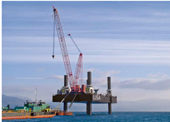
Figure 2: Jack-up construction vessel Smit Lisa, lifted, mention the gap between platform and water level; ref. www.smit.com
