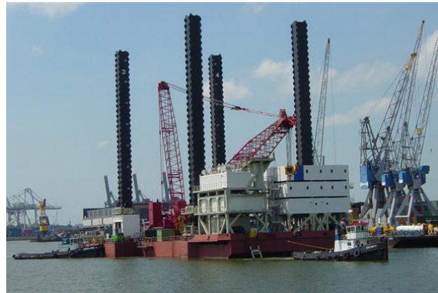
Figure 3: Smit Lisa, towed, mention the retracted legs; ref. www.tugspotters.com
