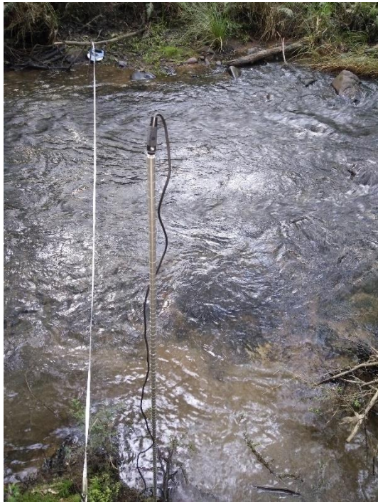
Figure C. 4: A picture of a flow velocity measurement being taken. The velocity meter is connected to the metal pipe, which is also show in the picture. The metal pipe is also used to determine the depth of the river.
