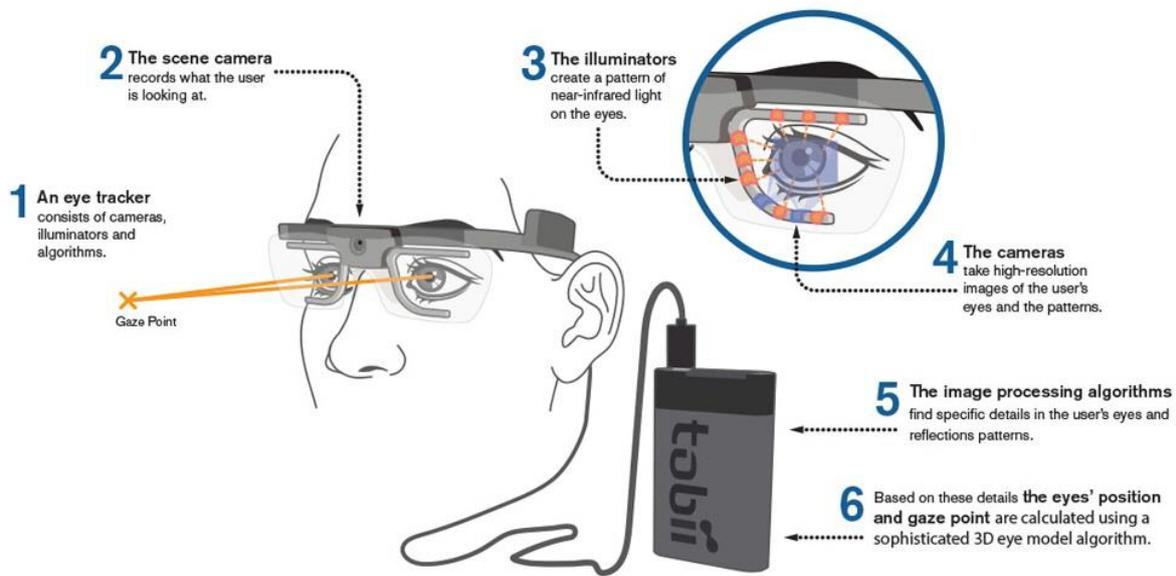
Figure D2: The working mechanism of a wearable Tobii Glasses Eye Tracker Device (2).
