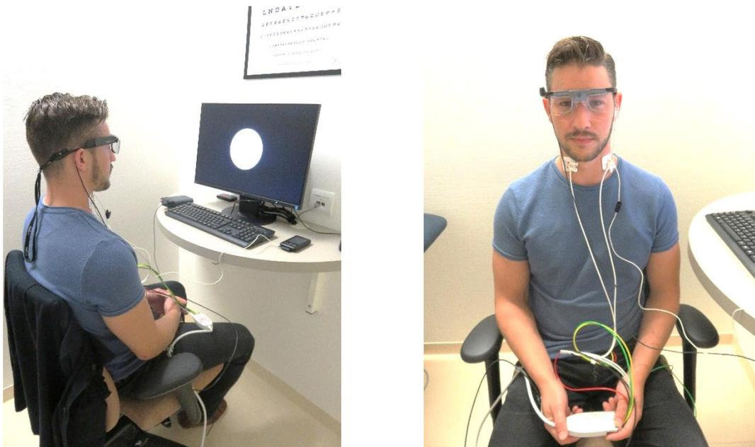
Figure C1: The measurement set-up for the measurements. The Tobii Glasses 2 Eye Tracker Device was placed on the subject's head. The ECG electrode were all applied. In this case it was a measurement with the tVNS, so electrode in the neck were place on both sides of the neck. Subjects sat in front of a computer screen situated at a distance of 50 cm.
