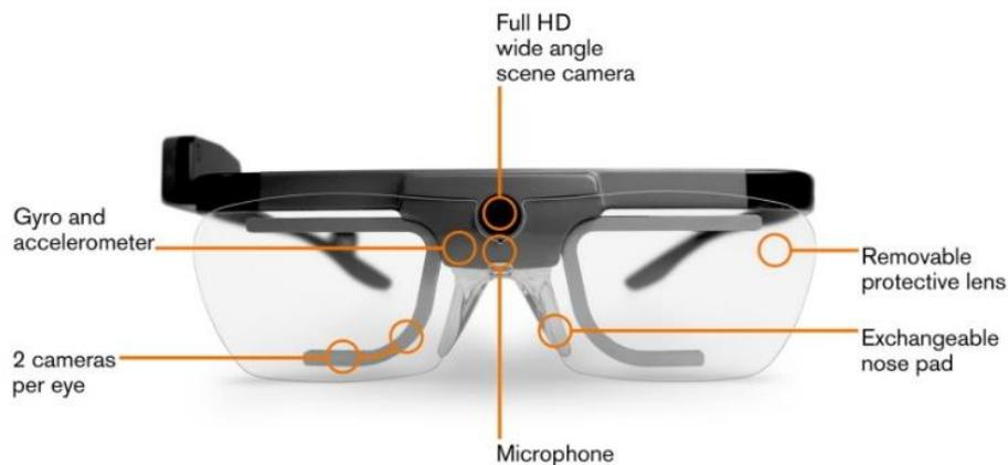
Figure D1: The Tobii Glasses Eye Tracker Device head unit (1).
