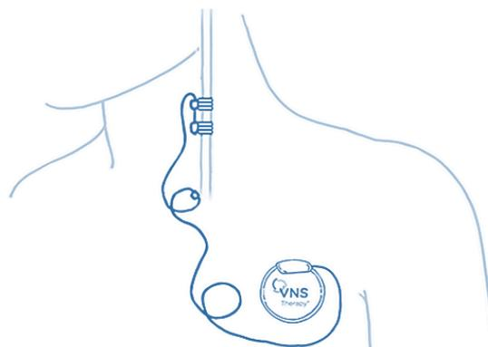
Figure 1: Schematic view of the electrode of the VNS wrapped around the vagus nerve (24).
