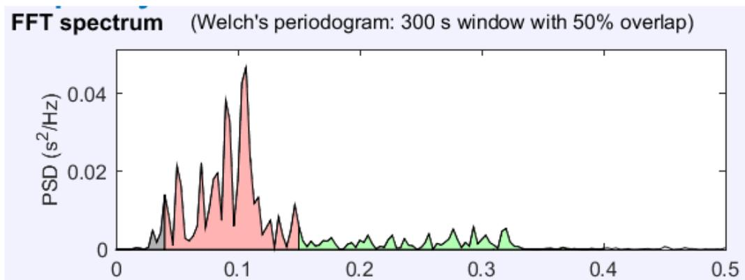
Table H3: This figure shows the obtained FFT spectrum, which was calculated with the non-parametric Welch's periodogram. The red area represents the LF and the green area represents the HF.
