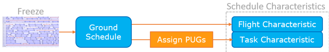
FIGURE 4.1: Process to calculate schedule characteristics in order to quantify a flight schedule (Freeze).
