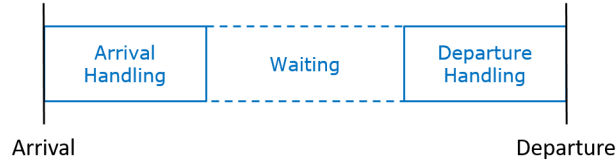
FIGURE 12.3: Phases of a single aircraft in the Arrival-Departure CTMC model including ground handling. The dashed waiting phase is optional.
